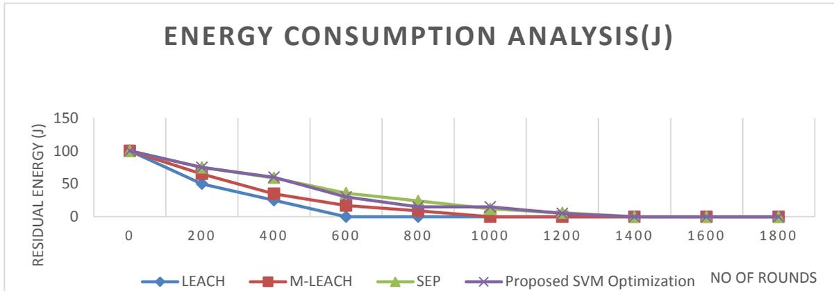
**Figure 2** Energy Consumption Analysis for the various protocols at Area of Dimension 60x120 Sq. meters (7200Sq.meters)
