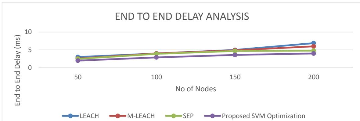
**Figure 5** End to End Delay comparison between the proposed routing protocols @Area Dimension 60x120Sq.meters
