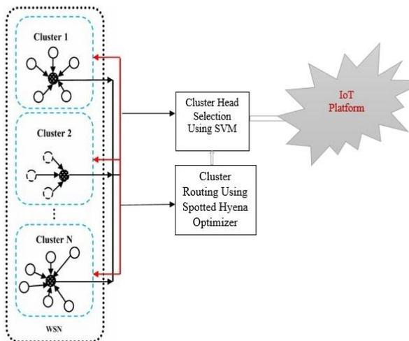
**Figure 1** Cluster Head selection for WSN using proposed Framework
