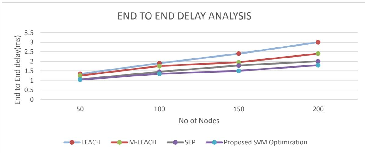
**Figure 6** End to End Delay comparison between the proposed routing protocols @Area Dimension 100x120Sq.meters.
